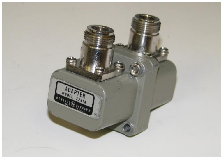
Figure 5.16: A cavity resonator using two HP X281A waveguide adapters.
