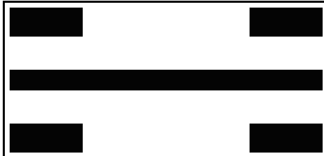
Figure C.3: Original "thru" board as measured for connector loss measurement and optimization (top layer).
